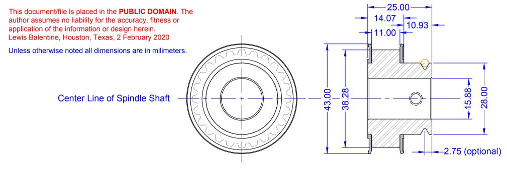
This is a modified set of XL 24 Tooth pullies to be used with a Taig Micro Lathe and a CS1000 Brushless DC motor. If you start with a pair of 15mm bore pullies then the only thing you need to do is size the bore of one for the 5/8 Taig spindle shaft.
